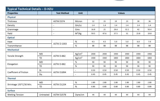
Storage and Handling: D-HZU needs to be stored in a closed warehouse below 35°C temperature and should not be exposed to direct sunlight, light sources and humidity. If the material is stored in the recommended conditions, it is suitable for use within 10 months from the date of shipment. Although it is a tough film, any kind of external pressure or shock can damage the film roll. Therefore, it is recommended to move the film roll with the help of proper equipment only.
