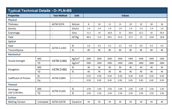
Storage and Handling: D-PLN-BS needs to be stored in a closed warehouse below 35°C temperature and should not be exposed to direct sunlight, light sources and humidity. If the material is stored in the recommended conditions, it is suitable for use within 10 months from the date of shipment. Although it is a tough film, any kind of external pressure or shock can damage the film roll. Therefore, it is recommended to move the film roll with the help of proper equipment only.
